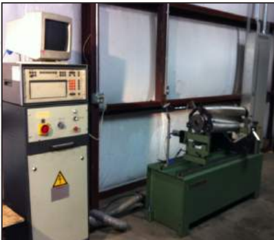
Roots Blower Scroll Precision Balancing
