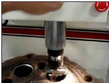
Machining, Re-Qualifying Cylinder Heads
