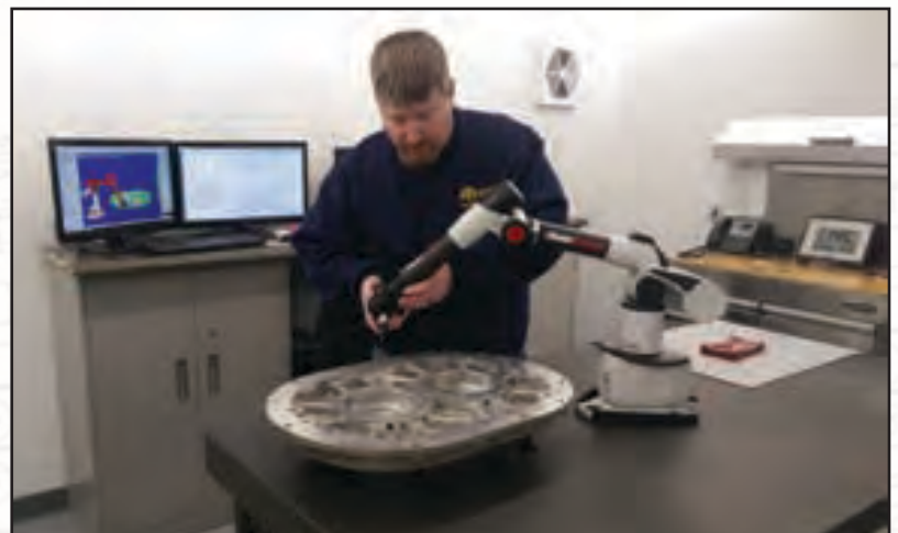
CMM Measuring for Accuracy
